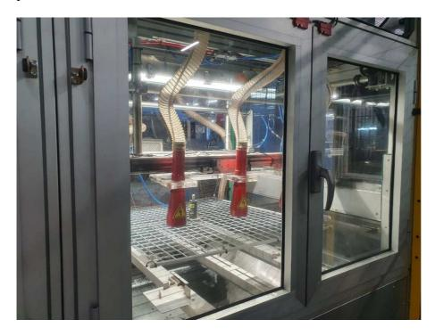
For profiles, the difficulties of flockability are multiplied by the fact that it is complex to reach the fibres evenly across the entire **section of** the profile. For this reason, it was decided to use the technique of electropneumatic flocking, which, by precisely mixing air and flock, allows the fibres to reach areas that are difficult to flock.
