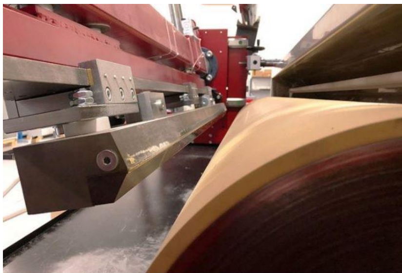
Image #7 - Application with industrial Slot-Dye
